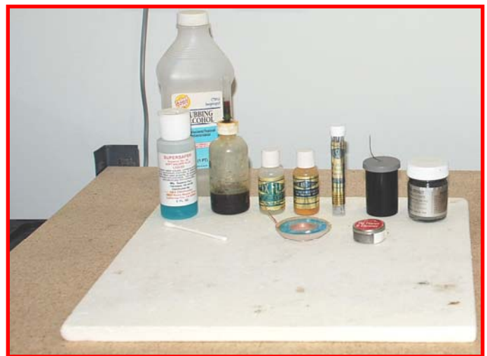
Photo Two: Ceramic Soldering Pad 12" x 12" (Withstands Temperatures to 2,800 degrees F) On Ceramic Soldering Pad:
