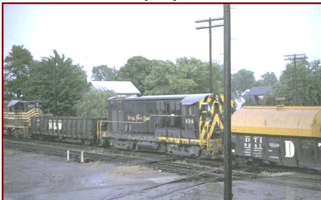
H-12-44 134 at Belevue OH - NKP Class FS-12a - Blt Nbr 12L721 - Blt 1953. Image © George Elwood
