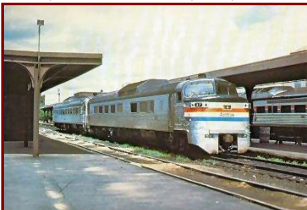
Modified Amtrak RDC-2 with Cowled Crew Safety Cab
