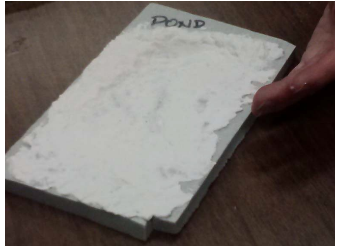
The Pond Base consists of a foam insulation board base that has been carved and covered with Sculptamold plaster
