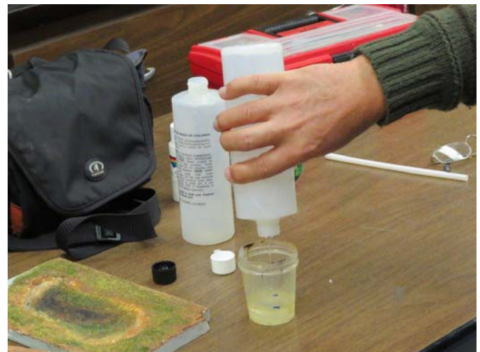
Pour equal amounts of resin & hardener into a plastic, glass or waxed paper container (not Styrofoam) and mix for 2 minutes
