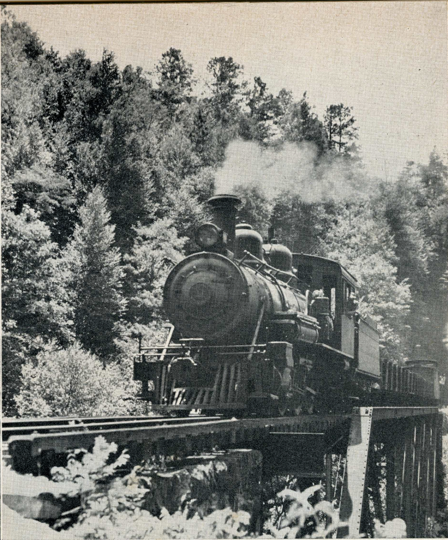
The Ten-Wheeler has just emerged from a tunnel, and the fireman and head brakeman are inspecting the train on the brief stretch of open track across this inverted truss bridge. The tunnel was approached at both ends by bridges; construction of the line through Doe River Gorge was not easy.
